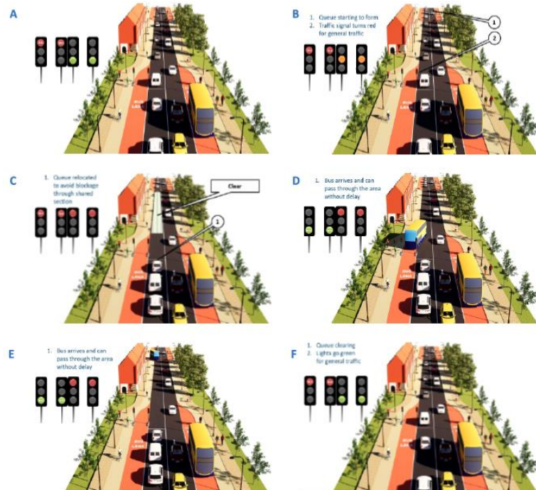
Figure 12-7 Bus Priority Signal Schematic Operation
